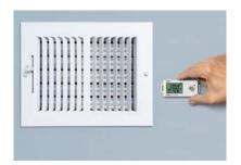
Stand-alone data loggers are compact and easy to set up and deploy. You have a choice of low-cost, standa-lone loggers with internal sensors for measurements at the logger location, or multi-channel loggers with external sensors for monitoring at some distance from the logger. All standalone loggers communicate with a PC or Mac via USB.
