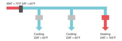
Historically, cooling systems without supply air temperature reset are designed and configured to deliver 55°F air without considering whether this temperature provides optimum performance or comfort. Further, building operators often respond to hot complaints by reducing supply air temperature (where possible) to satisfy one or two zones, but fail to realize the detrimental effect this may have on the balance of the system and occupants.
