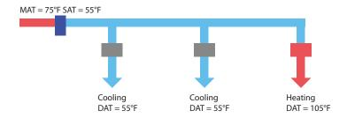
Raising the supply air temperature to 65°F (for example) reduces the amount of heating energy required at the last zone. In addition, the remaining zones are less likely to be overcooled because the discharge air temperature is higher.
