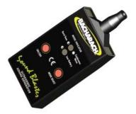
Some Tru Pointe<sup>®</sup> Ultra kits include Bacharach's ultrasonic sound generator, the SoundBlaster<sup>®</sup>. The SoundBlaster<sup>®</sup> is used to artificially pressurize items and detect potential leaks using a 115dB ultrasonic tone. The Tru Pointe<sup>®</sup> Ultra can detect the tone as it escapes in areas that are not under pressure.
