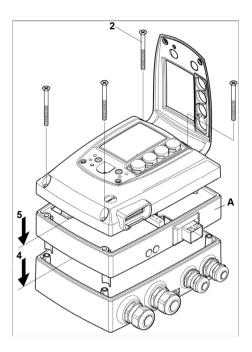
Place Ethernet module (A) on lower part of instrument (4). 4
