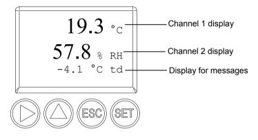
Four keys enable the user to navigate/scroll through the menus and enter/amend values and settings:
