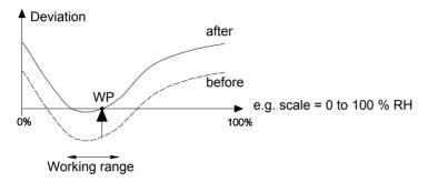
The advantage of the 1-point adjustment is the good measuring result in the working range. But the further away the measurement is from the working point, the greater the deviation can become. The 1-point adjustment should therefore only be used for a relatively narrow measuring range (working range), e.g. clean room applications, air conditioning applications for storage and similar.
