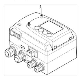
Loosen screw connection (1) of service flap and open the flap.
