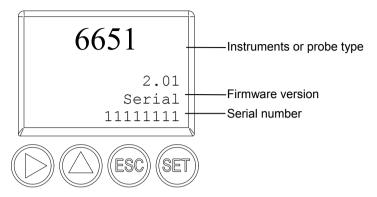
The serial numbers of the transmitter and probe can be read off.
