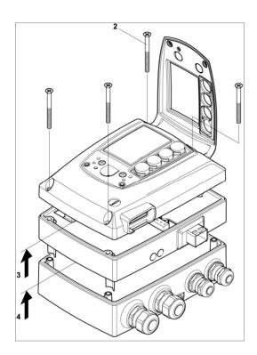
2 Loosen and remove housing screws (2).
