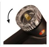
Remove particle filter (1) and store it to reinsert it after the measurement.
