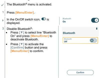
When the Bluetooth<sup>®</sup> icon is not shown on the display, Bluetooth<sup>®</sup> is switched off.
