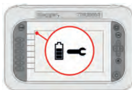
Current operational state. Currently in Setup operation
