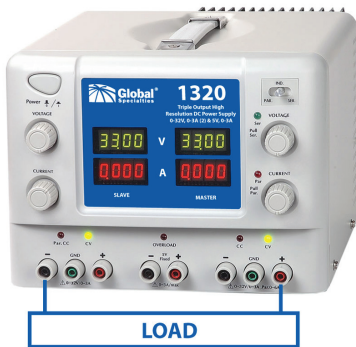
Figure 5. Series Tracking Mode
