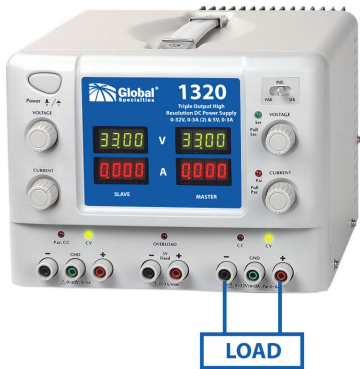
Figure 6. Parallel Tracking Mode
