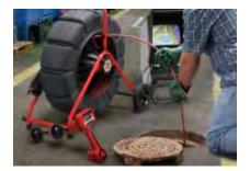
**1. Locate Cameras** Use Scout to locate your SeeSnake™ or other video inspection equipment. All SeeSnake Plus cameras come equipped with in-line transmitters.
