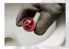
**3. Locate Flushable Transmitters** Use Scout to meet your septic and other locate needs. Scout quickly and accurately locates the RIDGID float sonde. Simply flush the float sonde and begin locating.
