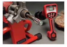
2. Locate Remote Transmitters Use Scout to extend the service provided by your drain cleaning machines. Simply attach a remote transmitter and begin mapping drain lines with Scout.
