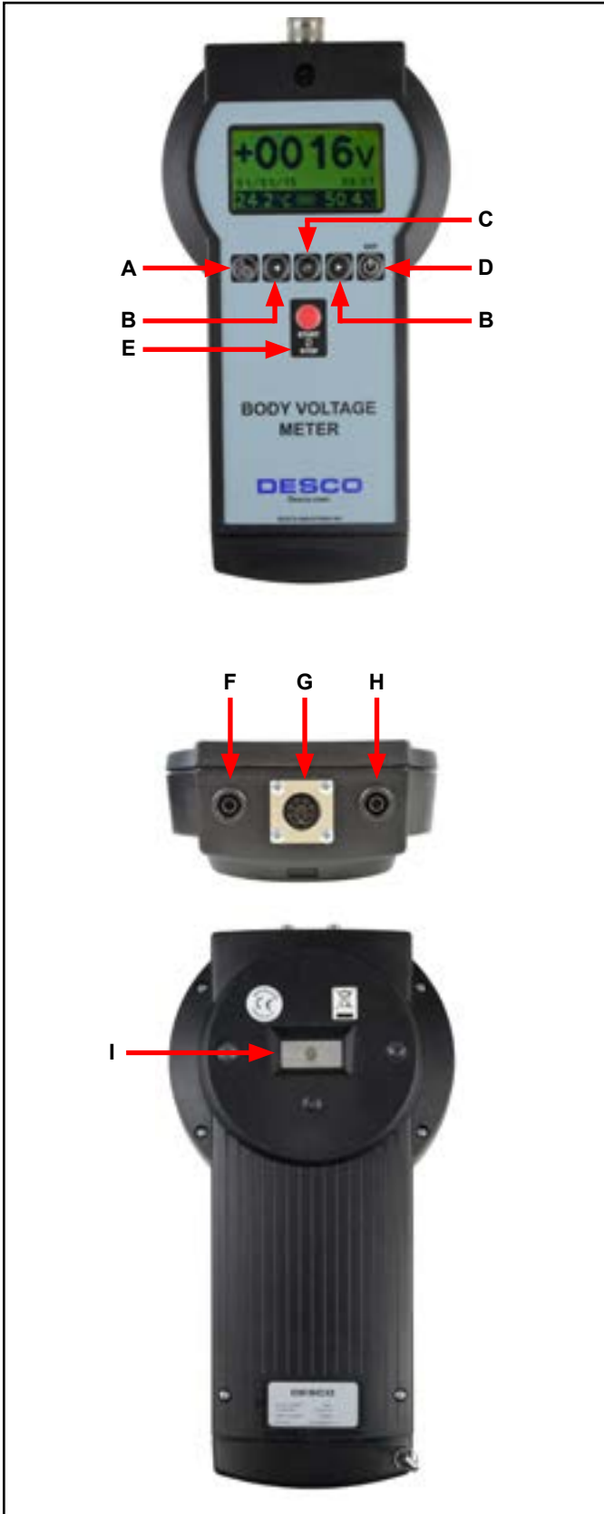
Figure 2. Body Voltage Meter features and components
