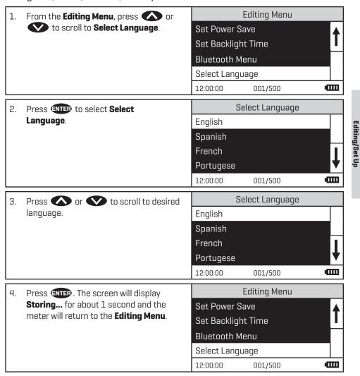
NOTE: If meter unintentionally switches to another language, use the procedure above to reset the meter to the desired language. For example, to reset the meter to English:
