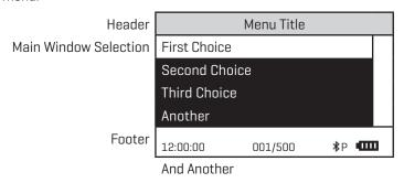
A light bar will indicate the menu choice. As the menu is scrolled through, the light bar will highlight different menu choices. Pressing the button will select the menu choice that is indicated by the light bar.
