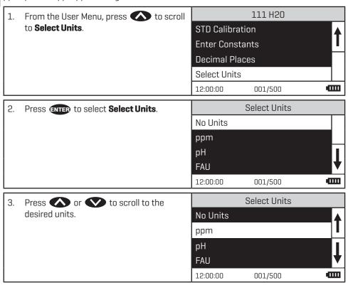
4. Press STEP to select the units. The screen will display **Storing...** for about 1 second and the meter will return to the **Edit Test** menu.
