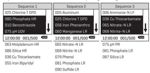
These alterable sequences allow a series of tests to be setup that are run frequently. The order of the individual tests in the sequence can be determined by the user. After running a test, press **ENTER** to select the next test in the sequence. Continue this pattern until the entire sequence has been completed.
