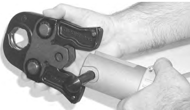
Figure 5 – Pulling The Jaw Set Mounting Pin Out
