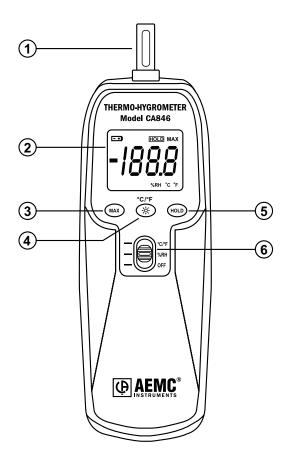
1. Temperature/humidity sensor with protective sensor cover
