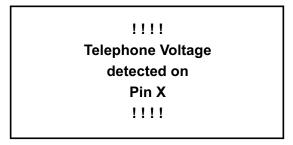
**NOTE:** The pin on the RJ45 connection, on which the voltage is detected, is displayed.
