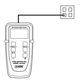
If a Telecom Network Voltage is present, the unit will give a continuous audible warning, and display the following:
