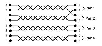
Message: Crossed Wires Pin 3 5 at Remote End or Near End
