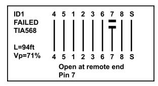
Notice the word **FAILED** under the cable ID1 and also the detailed message at the bottom of the display.
