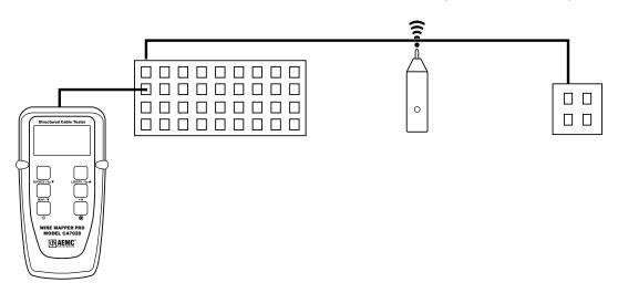
Pressing the ••••) key will inject a warbling (oscillating) tone into the cable or link under test. When set, the following will be displayed:
