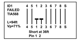
In this situation, the graphical portion of the display also shows that the fault is a short between pins 1 and 2 and the short is drawn at an approximation to the distance along the cable or link under test, at which it occurs.
