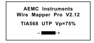
When the unit is first switched on, it will display the opening screen giving the software version and remaining battery capacity.
