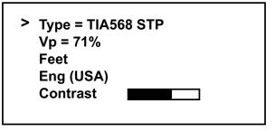
The > (line selector) is moved by pressing the MAP /  $\checkmark$  button. When the appropriate line is selected, the SERVICE / Vp  $\checkmark$  and LENGTH / Vp  $\blacktriangle$  buttons may be pressed to increment or decrement through the alternative options for the selected item.
