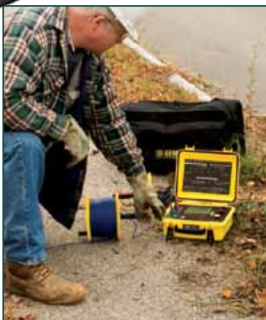
The Model 6470-B quickly checks ground rod resistance with its Connect – Press – Read approach.
