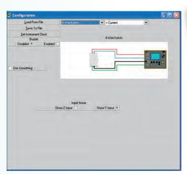
DataView software provides a convenient way to configure and control ground resistance tests from your computer. Through the use of clear and easy-to-use tabbed dialog boxes, all ground tester functions can be configured and tests can be initiated. Results can be displayed in real-time and stored in your PC. Reports may be printed along with the operator's comments and analysis.
