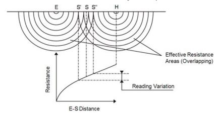
On the other hand, if the auxiliary potential rod S is located outside the effective resistance areas, as S is moved back and forth the reading variation is minimal. The readings taken should be relatively close to each other, and are the best values for the resistance to ground of the ground E. The readings should be plotted to ensure that they lie in a "plateau" region as shown below.
