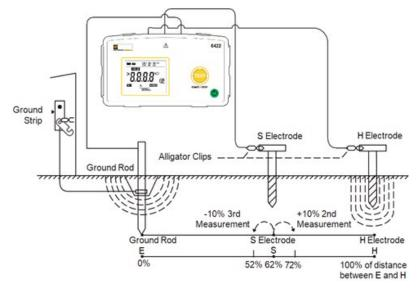
Consider the illustration below, which shows the effective resistance areas (concentric shells) of the ground electrode E and of the auxiliary current electrode H. The resistance areas overlap.
