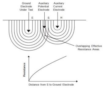
If readings were taken by moving the auxiliary potential electrode S towards either E or H, the reading differentials would be great and we could not obtain a reading within a reasonable band of tolerance. The sensitive areas overlap and act constantly to increase resistance as S is moved away from E.
