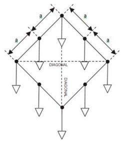
In multiple electrode systems, the 62 % method electrode spacing may no longer be applied directly. The distance of the auxiliary electrodes is now based on the maximum grid distance (e.g. in a square, the diagonal; in a line, the total length). A square having a side of 20 ft will have a diagonal of approximately 28 ft.
