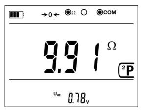
The instrument displays the measured value minus the compensation. The value displayed may be negative if the leads used for the measurement are not the ones that were compensated. In this case, repeat the compensation. Lead compensation is preserved after Auto Off but not after the instrument is manually turned OFF.
