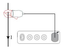
The measurement appears on the LCD.
