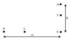
If the measurements match, they are valid. If they differ significantly, they could be influenced by factors such as ground currents or a groundwater artery. In this case, we recommend driving the auxiliary rods deeper into the ground.
