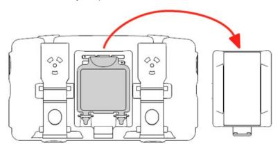
1. Pull open the rubber seal covering the battery compartment.
