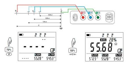
The instrument immediately calculates and displays the average of the three measurements and the percent difference between the lowest and highest values. For the measurement to be valid, the difference must not exceed 5 %. If it is, place the H electrode out further and repeat the tests at the 52 %, 62 %, and 72 % distances.
