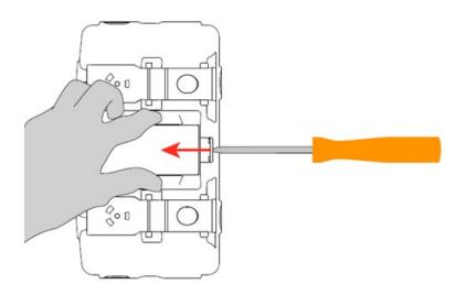
3. Remove the battery compartment cover.
