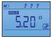
3 P mode used for measuring the grounding system. The resistance of the injector electrode and the test voltage are also displayed
