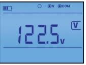
Live voltage is displayed when the V/A function is selected and test leads are connected to AC or DC voltage (Model 6424)
