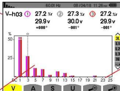
Display of 3 phases 3L, of L1, L2, L3, N, or of expert mode (three-phase connection only – see §6.5). To select the display press the ▲ or ▼ button.
