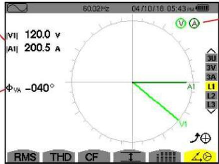
Indicators showing potential saturation of the channel.
