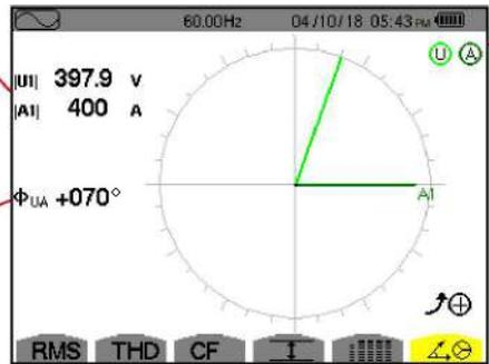
Indicators showing potential saturation of the channel.
