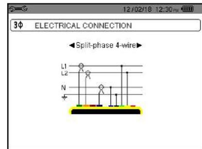
Figure 3-7 (4-wire split-phase connection)
