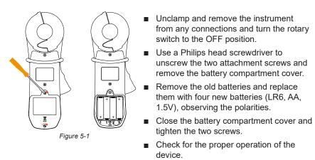
**NOTE:** The alkaline batteries can be replaced by NiCd or NiMh rechargeable batteries (AA, 1.2V) having similar characteristics. However, the time between the low battery message and the Auto Power OFF will be shorter with the rechargeable batteries.
