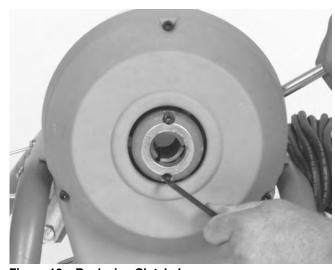
Figure 12 – Replacing Clutch Jaws
