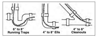
Figure 9 - Heavy Duty Cable Application
