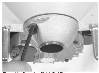
Figure 14 - Removing Clutch End Play
