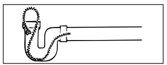
Figure 7 - Looping Cable In Line
