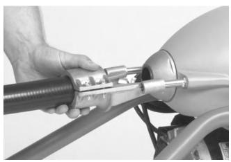
Figure 3 - Rear Guide Hose Attachment
