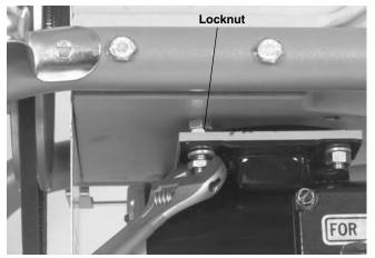
Figure 15 - Adjusting V-Belt Tension
