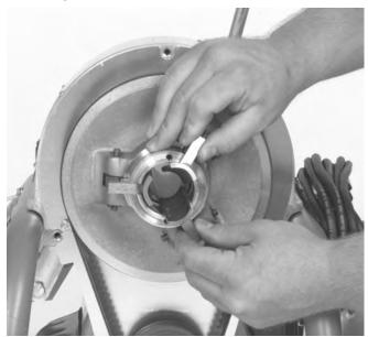
Figure 13 - Replacing Clutch Jaws
