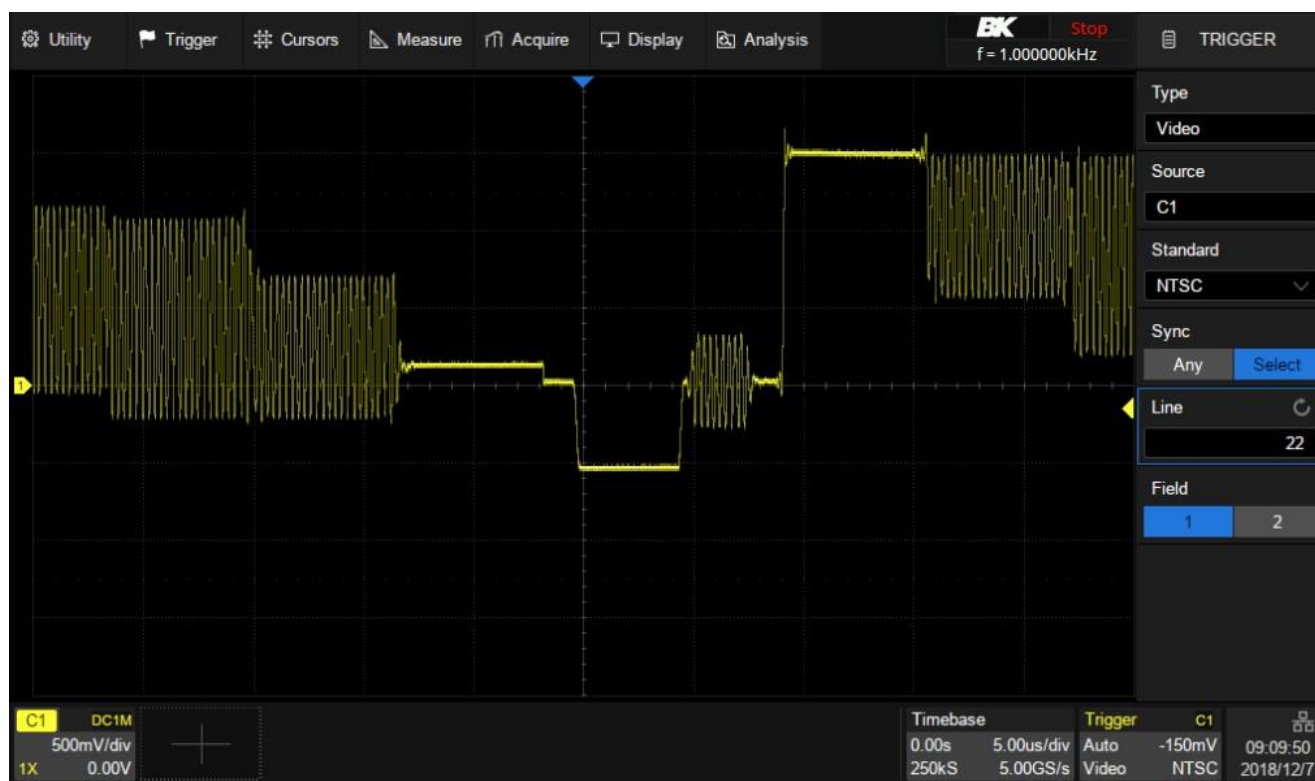
Figure 9.14 Triggering on a Specific Line of Video
