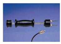
Two insulated pins with 1 <sup>1</sup>/<sub>16</sub>" penetration. Used to measure wood moisture content at various depths.
