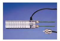
Two insulated pins with 3 ¼" penetration. Used for roofs, insulation, or EIFS.
