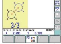
Determine each position (a1, a2, a3) on round hole A, following the measurement navigation procedure on the LCD.
