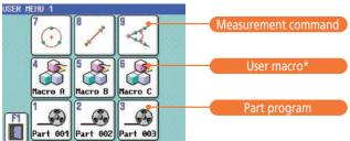
\* A user macro is a measurement command created by the user, and is a combination of several standard QM-Data200 measurement commands. Note: Up to three user menus, from [USER1] to [USER3], can be registered. A maximum of nine icons can be registered for one menu.
