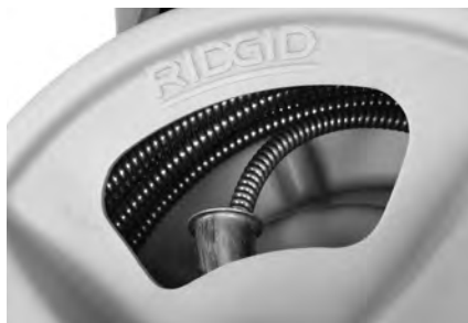
Figure 18 – Coil Cable Into Drum As Shown
