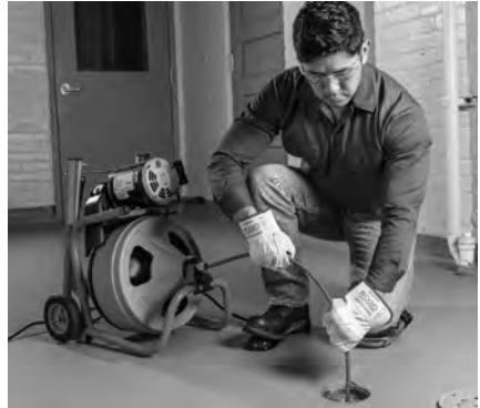
Figure 13 – In Operating Position, Manually Feeding Cable
