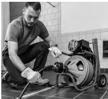
Figure 16 – Using Machine with Guide Hose
