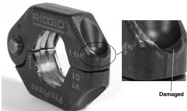
Figure 13 – Damaged Ring Pocket
