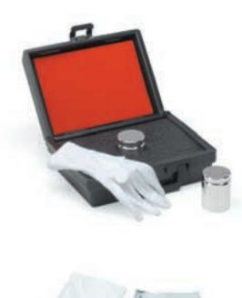
**Accessories** – Troemner can provide you with all the accessories you need to properly handle and protect your Electronic Balance Calibration Weights. A case and cotton glove are included for weights 10 g through 5 kg. Cases for larger weights are available at an additional cost. Please contact a Troemner sales representative for specific information on new cases, replacement cases, or special cases you need to store and protect your Electronic Balance Calibration Weights.
