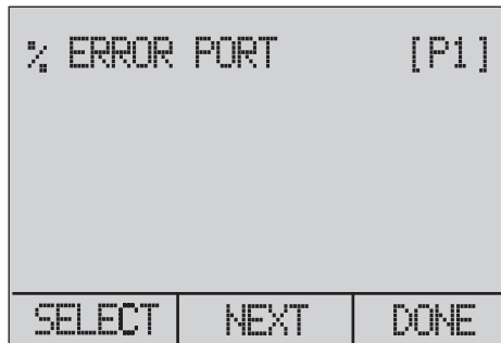
Figure 29. Port Setting Screen
