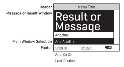
As described previously, the EXIT button allows an exit or escape from the current menu and a return to the previous menu. This allows a rapid exit from an inner menu to the main menu by repeatedly pushing the EXIT button. Pushing time will turn the colorimeter off.
