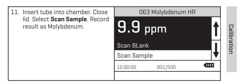
NOTE: The meter will remember the last scanned blank reading. It is not necessary to scan a blank each time the test is performed. To use the previous blank reading, instead of scanning a new one, scroll to Scan Sample and proceed. For the most accurate results, the meter should be blanked before each test and the same tube should be used for the blank and the reacted sample.
