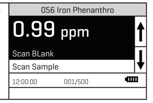
NOTE: The meter will remember the last scanned blank reading. It is not necessary to scan a blank each time the test is performed. To use the previous blank reading, instead of scanning a new one, scroll to Scan Sample and proceed. For the most accurate results, the meter should be blanked before each test and the same tube should be used for the blank and the reacted sample.
