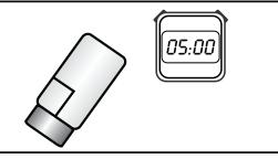
13. After 5 minutes insert tube into chamber. Close lid. Select **Scan Sample**. Record result as ppm Total Iron.
