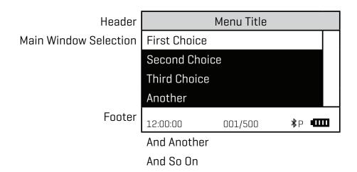
A light bar will indicate the menu choice. As the menu is scrolled through, the light bar will highlight different menu choices. Pressing the select the menu choice that is indicated by the light bar.
