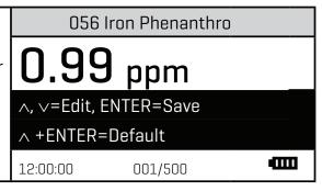
14. Press or to adjust the value shown to the concentration of the prepared standard, 1.00 in this example. NOTE: A maximum adjustment of 25% is possible.
