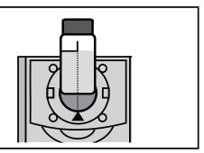
6. Remove tube from colorimeter. Add 6 drops of \*Acid Phenanthroline Indicator (2776).
