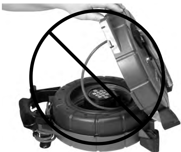
Figure 10 – Do Not Allow Cable to Uncoil Freely
