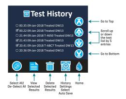
Logged results are viewed in Test History. Controls for viewing and managing single or multiple test records are located on the Test History screen. Tap the checkbox next to a test record to select it, then tap one of the buttons along the bottom to perform an action with the selected records.
