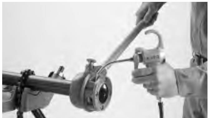
Figure 4 – Applying Thread Cutter Oil
