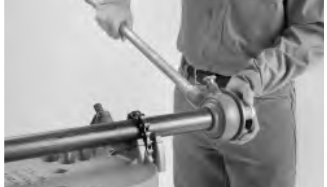
Figure 3 – Sliding Threader On Pipe
