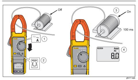
Figure 7. Inrush Current Measurement
