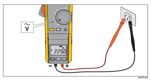
Figure 6. Measurement with Test Leads (AC Voltage Shown)
