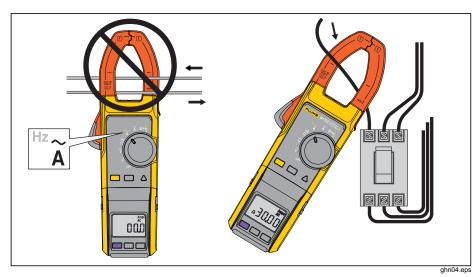
Figure 4. Current Measurement with Jaw
