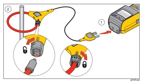
Figure 5. Flexible Current Probe Connection
