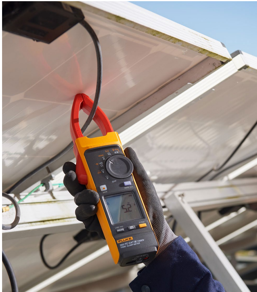
Measuring current on a PV panel with a Fluke 393 FC clamp meter.
