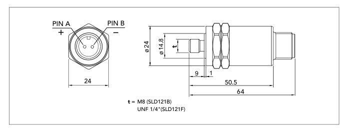
The vibration transducer SLD121B and SLD121F are piezoelectric accelerometers of compression type with built-in preamplifier, designed for vibration monitoring of industrial machinery. The electrical signal is isolated from the transducer housing.
