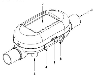
Figure 1-1 Model 4040/4043/4045 Mass Flowmeter
