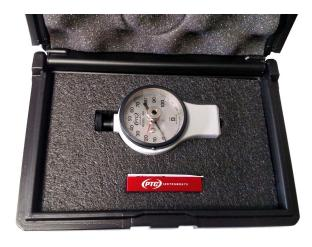
PTC Metrology™ is accredited by A2LA for durometer calibration to ISO/IEC 17025 & ANSI/NCSL Z540-1. NIST traceable certification is available for all durometer types covered by current ASTM D2240, ASTM F1957, ISO 868, ISO 7619 and DIN 5305 standards.
