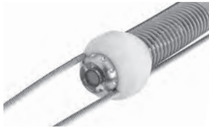
Figure 7 – Installing Guide On Camera Head
