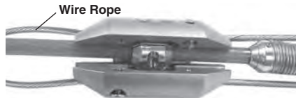
Figure 6 – Locate Pushrod Bulb In Shell
