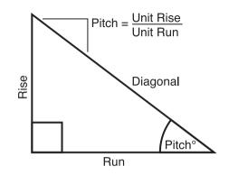
Using the Pythagorean theorem, the top row of keys on your Construction Master Pro will calculate instant solutions in dimensional format to right triangle problems (particularly, roof framing).
