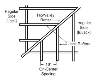
The *Construction Master Pro* uses the rise, run, diagonal, pitch and on-center spacing values to calculate *regular* and *irregular* hip/valley and jack rafter lengths (excluding wood thickness, etc.).
