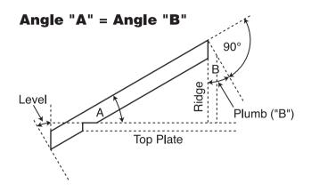
**Plumb:** Vertical Cut. The angle of cut from the edge of the board that allows the rafter to mate on the vertical side of the ridge rafter.
