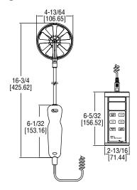
The MODEL 473B 100 mm Vane Thermo-Anemometer Test Instrument is a versatile unit that quickly and easily measures air velocity or volumetric air flow, as well as air temperature and humidity in imperial or metric units. A stainless steel 100 mm vane probe is included, which has a comfortable hand grip. The extruded aluminum housing fully protects electronics, yet is lightweight and comfortable to hold.
