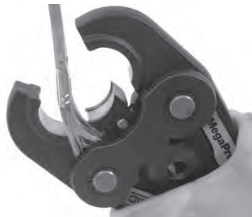
Figure 13 – Cleaning Segment Area of MegaPress Jaw
