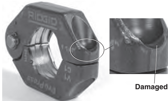
Figure 11 – Damaged Ring Pocket
