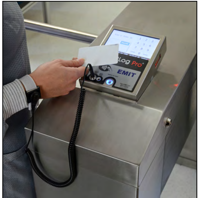
Figure 5. Holding a proximity badge in front of the RFID icon on the SmartLog Pro®
