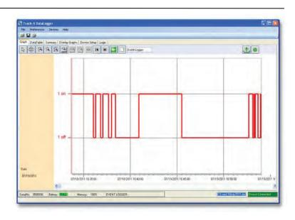
Software automatically calculates total time on, time off, and total test time. Valuable information about run time and power cycling is easily interpreted.
