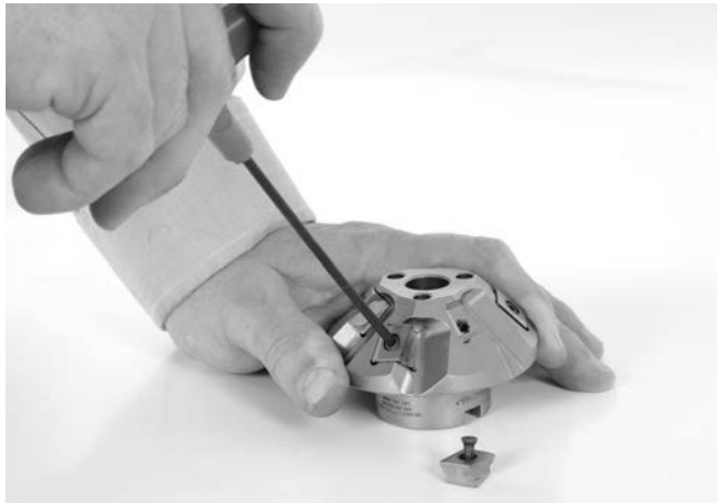
Figure 24 – Replacing Cutter Inserts
