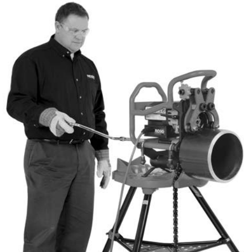
Figure 20C – Bevelling Operation (Fixed Beveller/Rotating Pipe)
