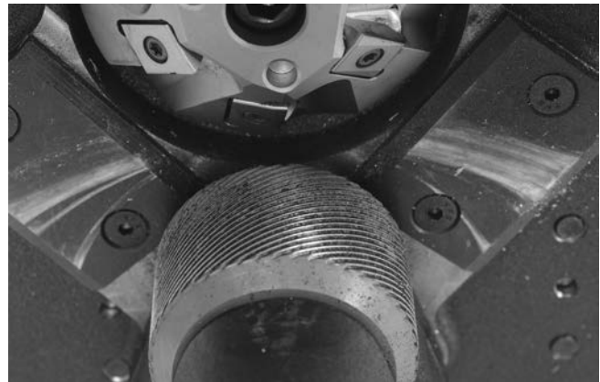
Figure 22– Clean Drive Roll Knurls
