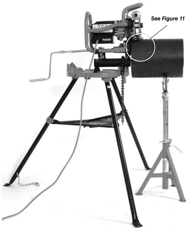
Figure 12 – Fixed Beveller, Short Pipe, One Pipe Stand
