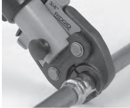
Figure 7 – Placing Scissor-Style Jaws Around Fitting
