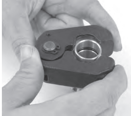
Figure 9 – Installing Press Ring onto Fitting
