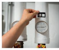
Attach  $\epsilon\text{-marker}$  and record the object with the digital camera in the thermal imager.
