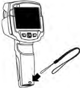
Figure 4 – Installing the lanyard
