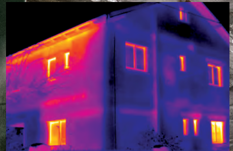
DETECT ENERGY LOSSES Immediately identify insulation voids and thermal bridges in building exteriors.
