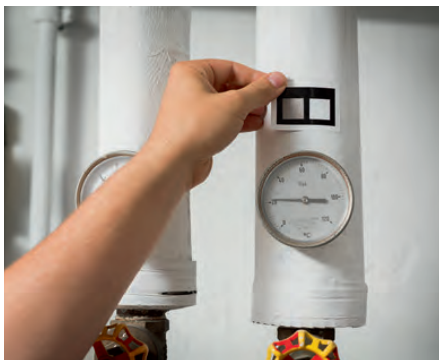
Attach E-marker and record the object with the digital camera in the thermal imager.
