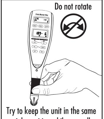
Try to keep the unit in the same upright position while you roll. Rotating the unit while rolling will add or subtract distance.
