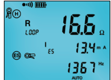
The 2 Clamp method displays clamp connection resistance, test current and frequency.
