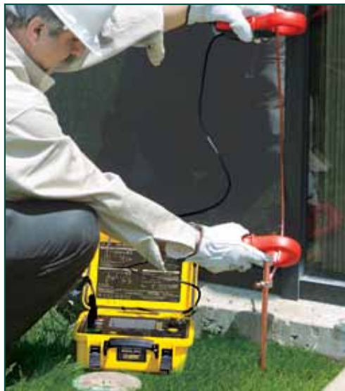
The Model 6471 performs a fast and easy way to measure the value of the earth/ground using the 2 Clamp method (no auxiliary rods needed).
