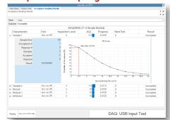
The MeasurLink® Acceptance Sampling feature calculates the correct number of samples to take and will reject or accept lots based on C=0 or ANSI Z1.4 standards. Display OC Curves for risk evaluation. Export to Excel or PDF.
