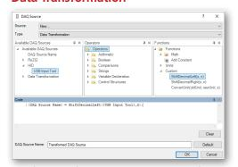
Transform data from measurement sources before storing and displaying results. This function can convert units and shift decimal points to make data collection even easier.
